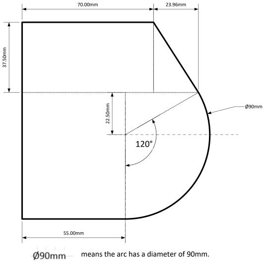
means the arc has a diameter of 90mm.
